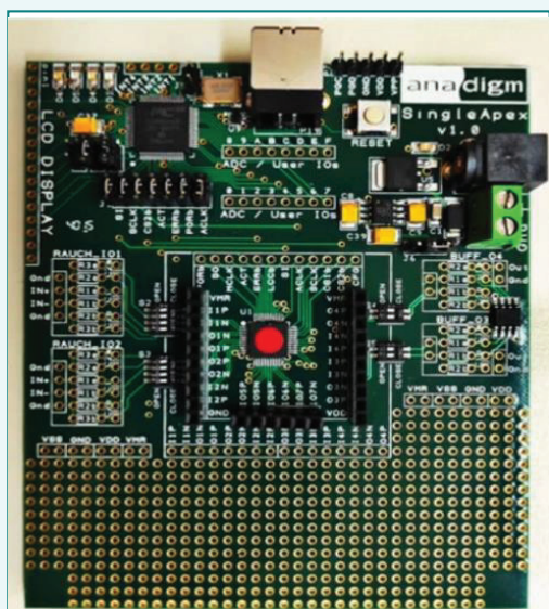
Anadigm SingleApex v1.0 AN231E04 development board
