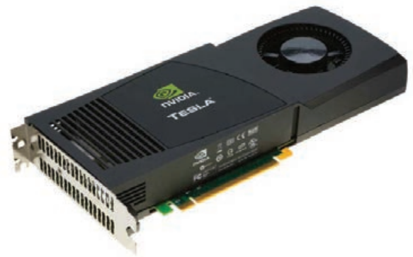
Fig 5: General Purpose GPU (GPGPU)
